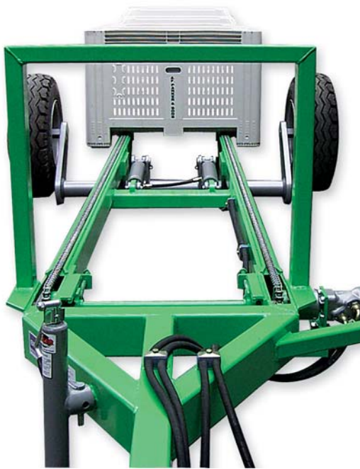
The Bin Loader 5000 loading with the axle dropped.
